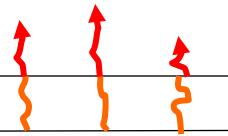
Strains concentrated above cracks in layer below
